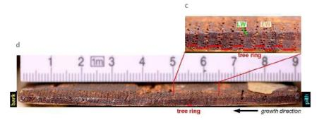
Fig.2. a) Cross-section of an oak trunk showing the tree's structure (see labels) and differently cut planks of (A) quarter (radial), (B) plain (tangential) orientation (red transparent bars). Annual tree rings of b) a softwood (spruce) and c) a hardwood (oak) species.
